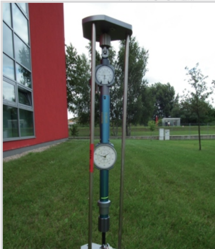
Mechanical distimeter ETH for specially precise measuring of deformations (dilatation, stress in structures, ...)
