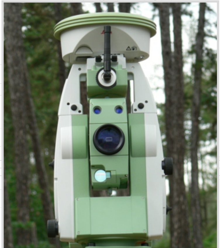
Robotized total stations Leica TCRP 1201+, TCRA 1201, TCRA 1101, TCRA 1105+ a TCR 705 auto
